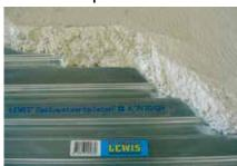
For best results use a C20/25 fine grade concrete (12 mm max aggregate) or a free flowing self-levelling anhydrite or cement based screed. Experienced screeding specialists may recommend the use of specific performance related screeds.
